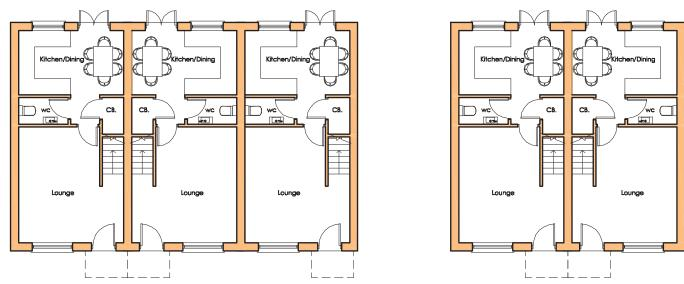
TYPE E (2B4P) - GROUND FLOOR PLAN (EITHER TERRACE OR SEMI DETACHED)
