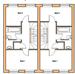
TYPE F - 3 STOREY, 3 BED - FIRST FLOOR PLAN (EITHER TERRACE OR SEMI DETACHED)
